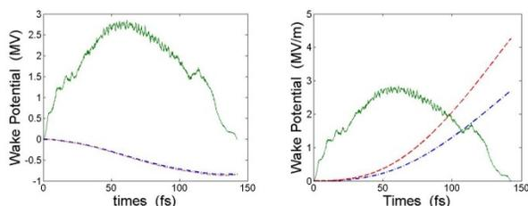
Figure 7: Longitudinal wake potential (left) and transverse wake potential (right) of peak current 3kA (green line). Blue line shows the results of rectangle constant-impedance structure, and red line shows the results of rectangle constant-gradient structure.
