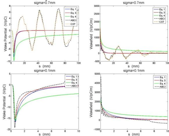
Figure 3: Longitudinal wake potential and wakefields of example cell at 0.7 mm and 0.1 mm rms bunch lengths.
