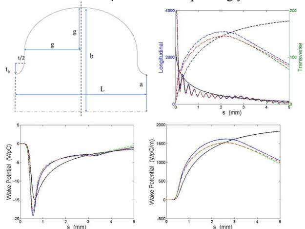
Figure 5: Optimized cavity and its wake function.
