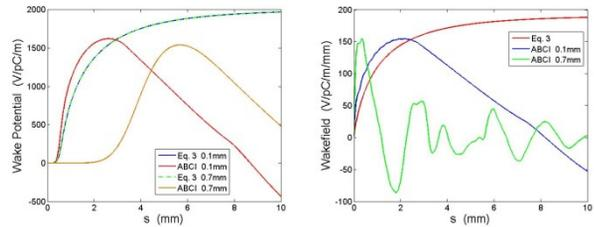
Figure 4: Transverse wake potential and wakefields of example cell at 0.1 mm rms bunch lengths.
