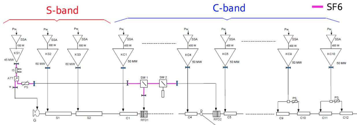
Figure 1: ELI-NP RF power generation and distribution system. 3 power units are used for the S-band injector, 10 units for the C-band booster. In magenta the two sections of sulfur-hexafluoride (SF<sub>6</sub>) components (isolator, attenuators, phase shifters and RF-switches) are highlighted.
