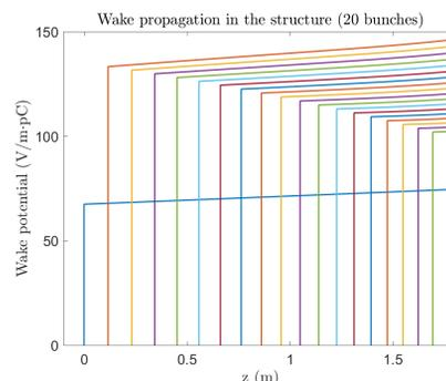
Figure 2: Snapshot of 20 wakes propagating within the TW C-band structure.
