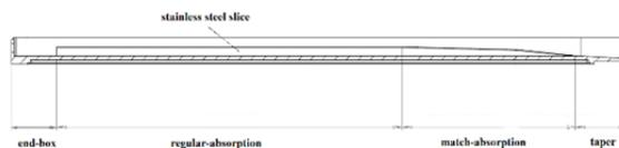
Figure 2: Sections of the load.
