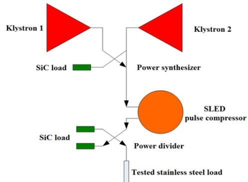
Figure 7: Constitutional diagram of test system.
