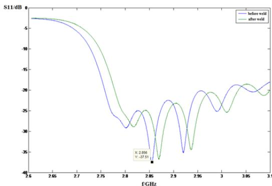
Figure 6: S-parameter before and after weld.
