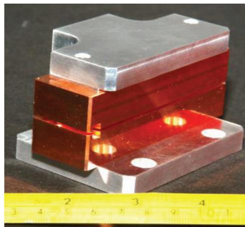
Figure 3: SLAC open mm-wave travelling wave accelerating structure.
