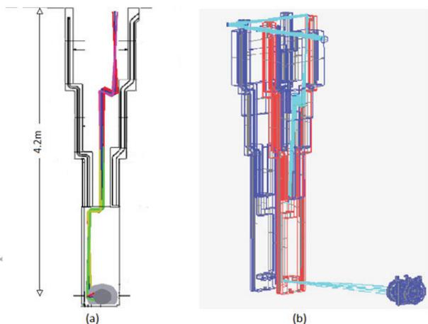
Figure 2: Optical Path from the PBW, inside the PBIP. (a) ZEMAX Implementation of original sketch design, superimposed onto a CAD drawing. Colours indicate rays from different object fields. (b) CAD wireframe model with highlighted PBW 'slice' (red) showing its optical path (blue).
