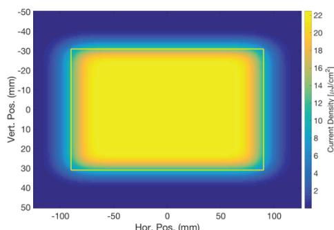
Figure 1: Beam on Target image simulation. Colour scale indicates the current density. The yellow rectangle shows the footprint enclosing a 99.9% beam fraction.
