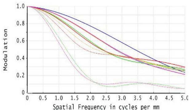
Figure 4: MTF Plot of full PBW optical system. Colours denote different Object field points. Broken lines show the blur in a vertical pattern, full lines in the horizontal.
