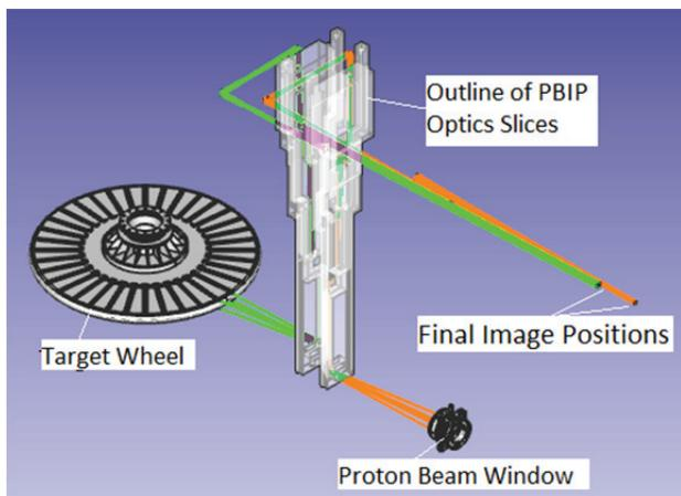
Figure 3: CAD view, with Zemax models of the PBW (red) and Target (green) system end-to-end optical paths. Only the target wheel, PBIP & PBW are shown; for clarity other structures around the target monolith are omitted.
