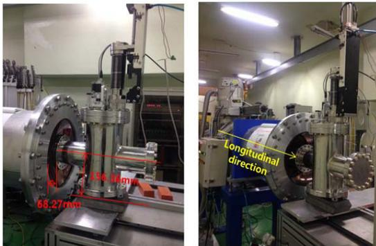
Figure 7: the picture of MC50 beam line and scintillation screen monitor.
