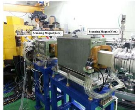
Figure 9: Picture of scanning magnet.
