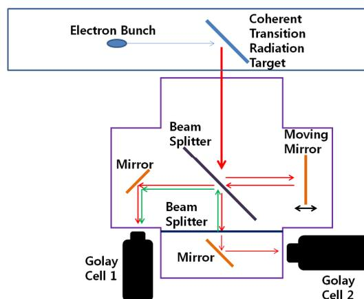
Figure 1: Michelson Interferometer's setup used in our experiment.
