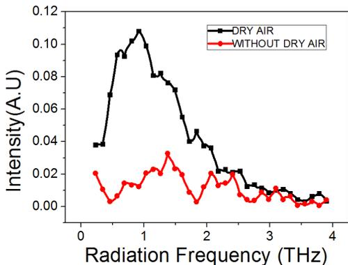
Figure 8: THz band with dry air and without dry air.
