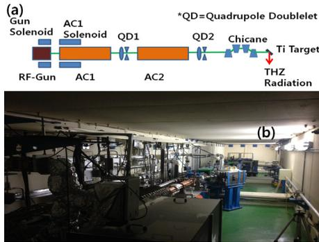
Figure 2: (a) Schematic Layout of the fs-THz linac and (b) a view of the fs-THz linac tunnel.
