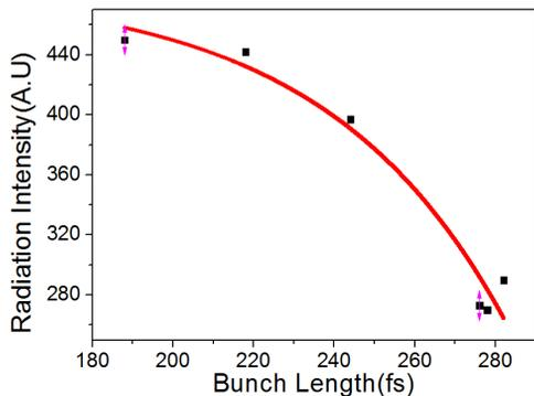
Figure 6: Bunch length versus THz radiation intensity.
