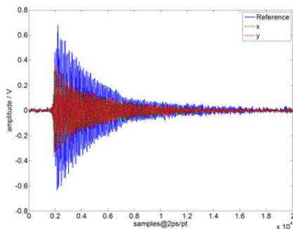
Figure 5: RF signals waveform of CBPM.
