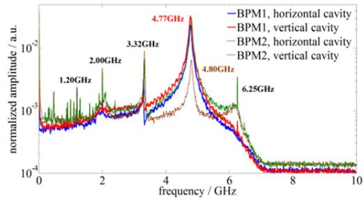
Figure 7: The spectrum of the position cavity.
