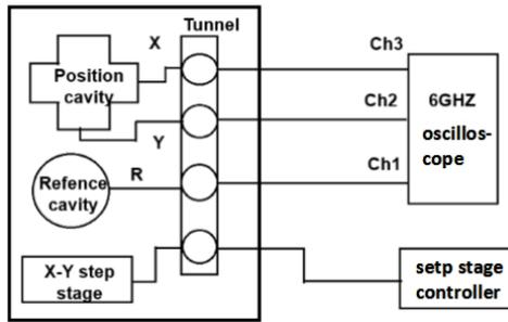
Figure 9: Diagram of the calibration system.
