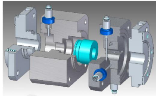
Figure 1: Three-dimension structure of the low Q CBPM.
