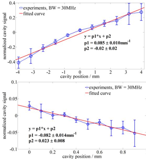
Figure 10: Calibration factors in horizontal (up) and vertical (down).
