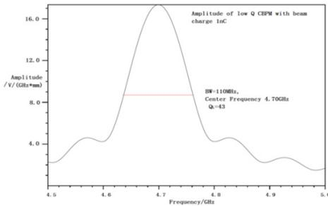
Figure 4: MAFIA simulation of the Q and central frequency.
