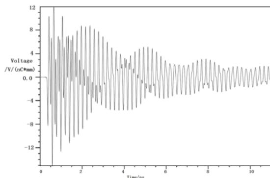
Figure 2: MAFIA simulation of the RF signals waveform.
