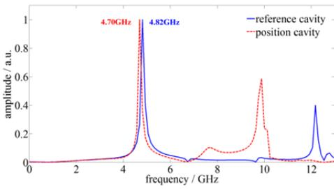
Figure 3: MAFIA simulation of the RF signals spectrum.
