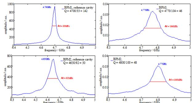
Figure 8: Q values of the two CBPMs ref cavity (left) and position cavity (right).
