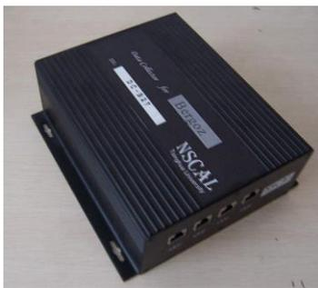
Figure 5: DAQ device for beam loss monitoring
