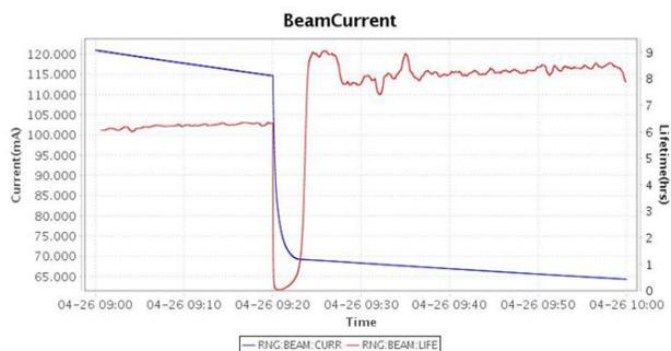
Figure 9: The beam current and life when beam lost at 9:20 on April 26, 2015.
