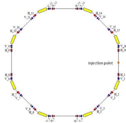
Figure 1: The layout of beam loss monitors in the HLS II storage ring.
