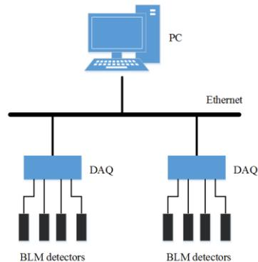
Figure 3: Beam loss monitor system structure diagram.
