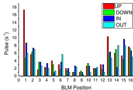
Figure 7: Beam loss distribution when beam can't be injected into storage ring at 16:05:53 17 April 2015.
