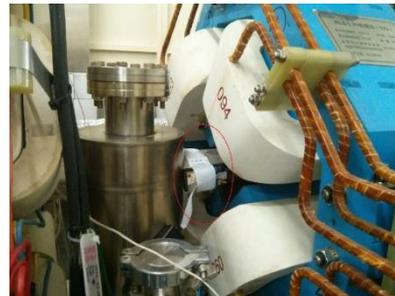
Figure 2: Site installation diagram for beam loss monitors in the HLS II storage ring.
