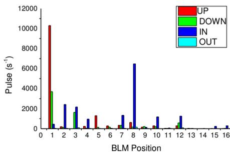
Figure 10: Beam loss distribution when beam lost at 9:20 on April 26, 2015.
