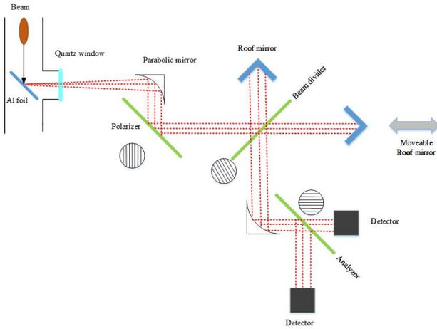
Figure 2: Concept design of the MPI for bunch length measurement.
