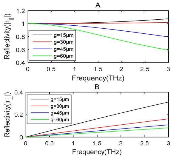
Figure 3: Calculated reflectivity for the parallel and vertical components of an incident electric field on a wire of  $10\ \mu\text{m}$  thickness grid with different  $g$ .
