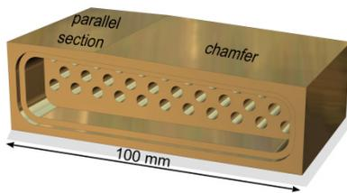
Figure 2: Schematic of the scraper brackets geometry.
