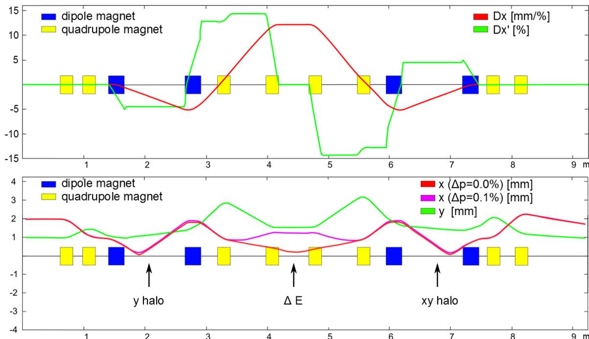
Figure 4: Beam dynamics calculation: The upper graphic shows the dispersion and its derivative along the new beam line. The beam envelope ( $1\sigma$  radius) for  $\Delta p = 0\%$  and  $\Delta p = 0.1\%$  is plotted below. The locations of the energy defining scraper ( $\Delta E$ ) and the halo scrapers are indicated by small arrows.
