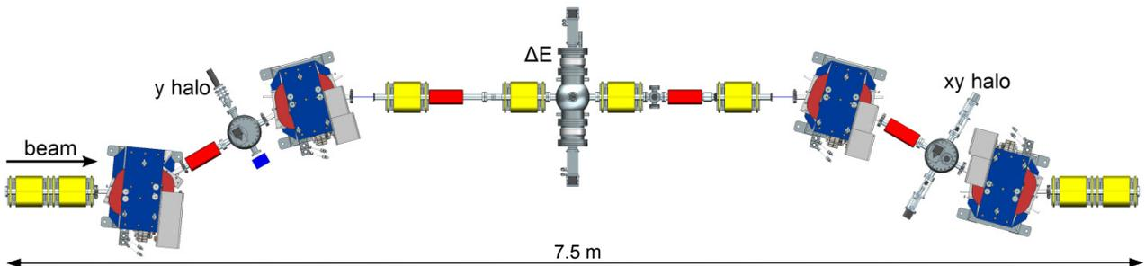
Figure 3: The high energy scrapersystem: from left to right the chambers for y halo-, energy defining- and xy halo-scraper can be seen.
