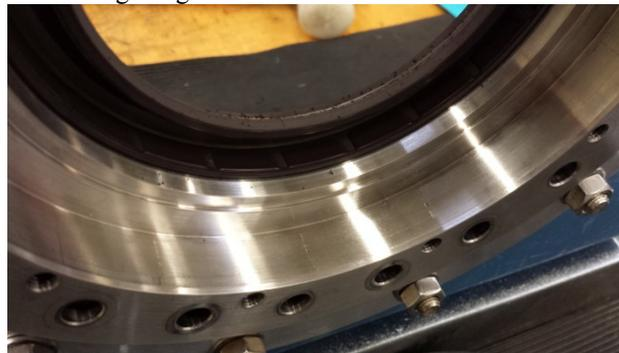
Figure 6: Damaged seal after some tens of dry turns.
