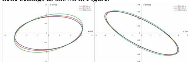
Figure 7: Comparing the horizontal and vertical emittance of a 1.4 MeV/u  $Ar^{9+}$  beam in front of the doublet measured with ROSE and existing scanners for different quadrupole settings.
