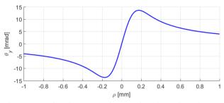
Figure 2: Deflection angle  $\theta_y$  as a function of the impact parameter  $\rho$  for 1 ps bunch RMS length and 100 µm transverse RMS size.
