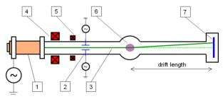
Figure 4: Diagnostic layout: 1 - electron gun, 2 - horizon-tal deflecting plates, 3 - probe electron beam, 4 - focusing solenoid, 5 - magnetic correctors, 6 - electron bunch, 7 - observation screen.
