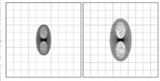
Figure 6: The probe electron beam images on the observation screen for 2 (left) and 1 ps (right) long bunch; grid size is 2 mm.
