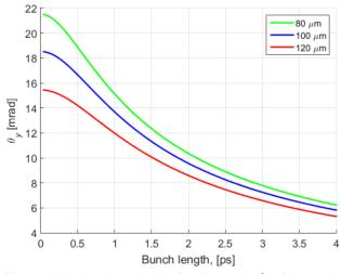
Figure 3: Maximal vertical deflection angle  $\theta_y$  of the probe electrons as a function of the bunch length for three transverse bunch sizes 80, 100 and 120  $\mu$ m.
