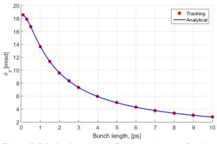
Figure 5: Maximal vertical deflection angle as a function of the bunch length according to Eq. 1 - blue curve and according to the particle tracking simulation – red dots.
