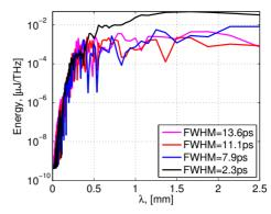
Figure 7: CTR spectrums the different bunches profiles shown on figure 4.
