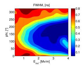
Figure 2: Full width at half of maximum of the bunch for the sub-harmonic buncher phase and maximum field.
