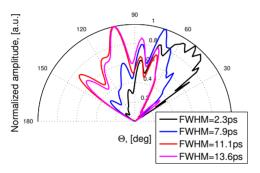
Figure 6: Coherent Smith-Purcell spectrum as a function of the observation angle for different maximum field in the FB. The grating used for these simulations has a pitch of 8 mm and a blaze angle of  $30^{\circ}$ . The upper figure gives the energy distribution, the lower figure is normalized so that the maximum amplitude of each line is 1.
