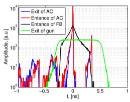
Figure 3: Longitudinal bunch size at exit of gun (FWHM=800 ps), at the entrance of FB (FWHM=92 ps), at the entrance (FWHM=2.35ps) and at the exit (FWHM=2.29ps) of the AC.
