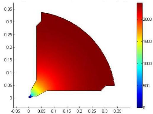
Figure 2: H-Field for RFQ cross section.
