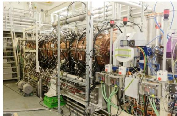
Figure 8: SPIRAL2 RFQ ready for conditioning.
