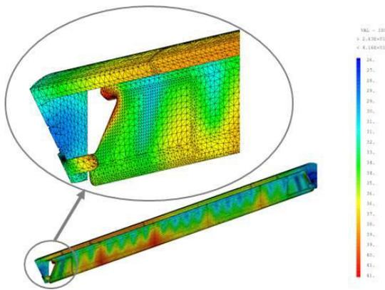
Figure 4: RF induced heating.
