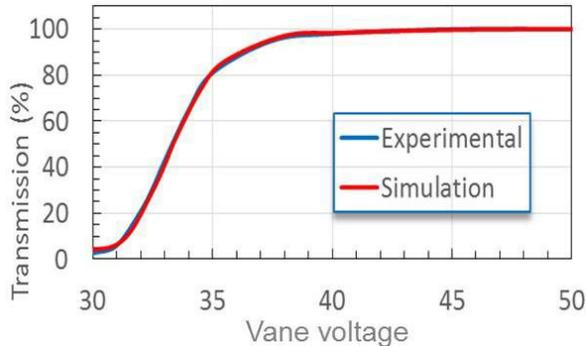
Figure 10: RFQ transmission vs vane voltage.
