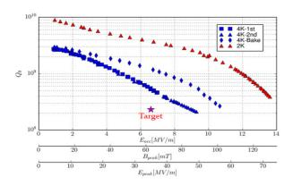
Figure 7: Measured Q factor of the QWR bare cavity measured before and after baking. After baking, the measurements were performed at 4K and 2K. The target value of Q factor at the operating condition is also given.
