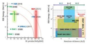
Figure 3: Characteristics of RISP. RISP will provide RIBs with energies ranging from tens of keV to intermediate energies of around 200MeV/nucleon with a high intensity and neutron richness. (FAIR and FRS in GSI, Germany; ISAC I and II in TRIUMF, Canada; RIBF in RIKEN, Japan; SPIRAL2 in GANIL, France; FRIB in MSU, USA.)
