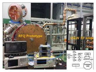
Figure 6: Photo of the prototype RFQ connected to the 15kW RF power amplifier. Insets display a segment of the RFQ fabricated as prototype (upper-left) and the block diagram of the RF power circuit starting from a signal generator (lower-right).
