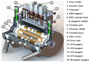
Figure 5: Schematic view of the 28-GHz superconducting EC-RIS. Only SC magnets and the cryostat is shown. The cylindrical plasma chamber, not shown here, is made of aluminium, 147 mm in diameter and 500 mm in mirror length (V<sub>plasma</sub>~85L) [2].
