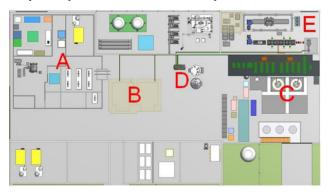
Figure 8: Layout of the SRF test facility. The area indicted by A, B, C and D are the main utilities of the facility: (A) Clean room for surface processing SC cavities; (B) Horizontal test area for cryomodules; (C) Vertical test area for cavities; (D) Cold box, liquid reservoir, distribution box (main components of 330W He cryoplant); (E) Area for installing the demonstration system.
