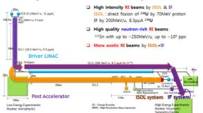
Figure 2: Schematic view of RAON. The operation modes, namely flow of driving beams for RI production, are shown.
