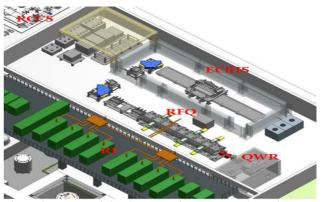
Figure 9: Layout of the demonstration system. The main components of the system was named; ECRIS, RFQ, and a single cavity cryomodule of QWR. The resonance control cooling system (RCCS) for the RFQ is shown partly in the upper-left side of the area.
