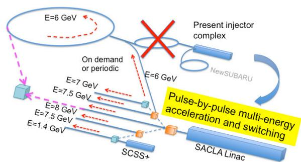
Figure 2: Schematic drawing of the SPring-8 accelerator complex after upgrading of SPring-8.
