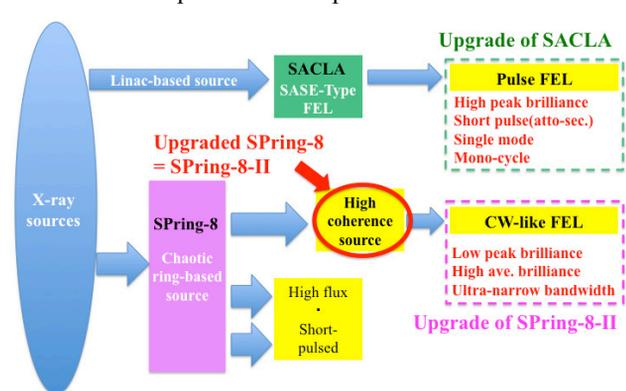
Figure 1: Schematic chart of X-ray source evolution and the SPring-8's strategy for the light source upgrade.
