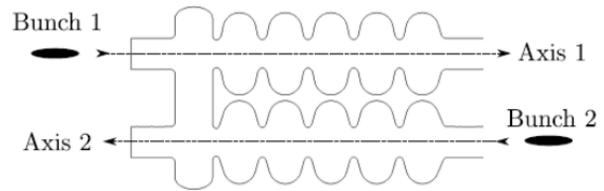
Figure 2: Schematic of dual axis cavity with accelerating (axis 1) and decelerating (axis 2) sections linked by resonant coupling cell.
