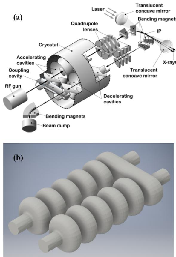
Figure 1: (a) Schematic of source of coherent radiation driven by SCRf dual axis asymmetric ERL. (b) Layout of dual axis asymmetric cavity for ERL.
