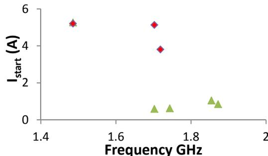
Figure 6: Comparison of HOMs start currents for ERL with asymmetric (diamond points) and symmetric (triangular points) cavities.
