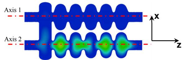
Figure 4: Contour plot (electric field) of one of the cavity HOM.
