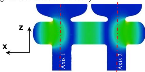
Figure 5: Contour plot of a typical HOM of the resonance coupler which is localised inside the coupler.
