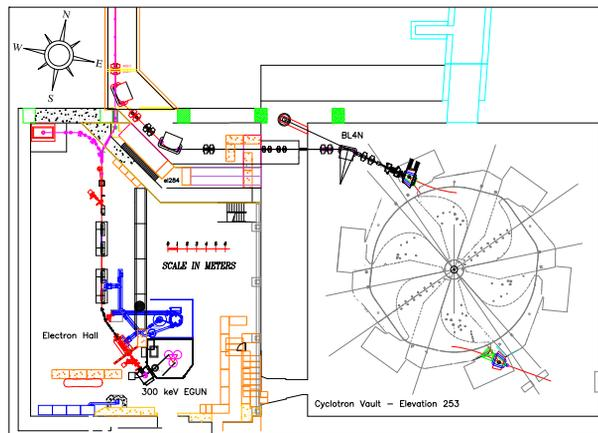
Figure 1: Schematic view showing the location of the electron linac (left) w.r.t. the 500 MeV cyclotron (right). The electron beam plane is ~61 cm (24 inches) below the cyclotron mid-plane in the electron hall.
