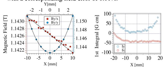
Figure 5: (Left) Transverse (red dots) and vertical (blue dots) peak field distribution. (Right) Vertical (blue dots) and horizontal (red dots) first field integrals.
