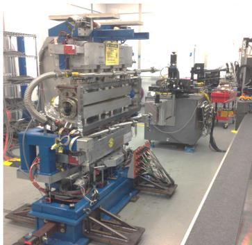
Figure 7: In-Vacuum Undulator X25.
