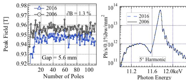
Figure 8: (Left) Comparison of the peak field distribution measured in 2006 (black dots) and in 2016 (blue dots). (Right) Comparison of the on-axis flux intensity calculated from the magnetic measurement in 2006 (black line) and in 2016 (dashed blue line).
