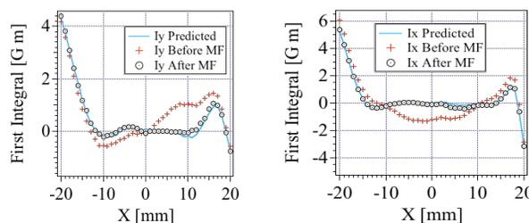
Figure 9: Comparison between measured field integrals before and after MF corrections and the “IDBuilder” predictions
