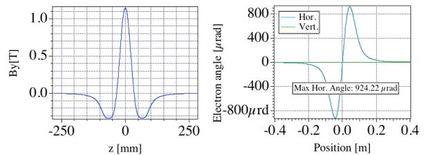
Figure 4: (Left) Vertical magnetic field on-axis. (Right) Vertical (green line) and horizontal (blue line) electron angle.
