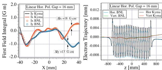
Figure 2: (Left) Comparison of the first field integrals between Kyma (solid lines) and BNL (dotted lines) at 16 mm gap and phase 0. (Right) Comparison of the 3 GeV electron trajectory using the measured magnetic field.
