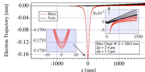
Figure 6: Horizontal (red line) and vertical (black line) electron trajectory off-axis measured at different X positions in the range  $\pm 10$  mm.
