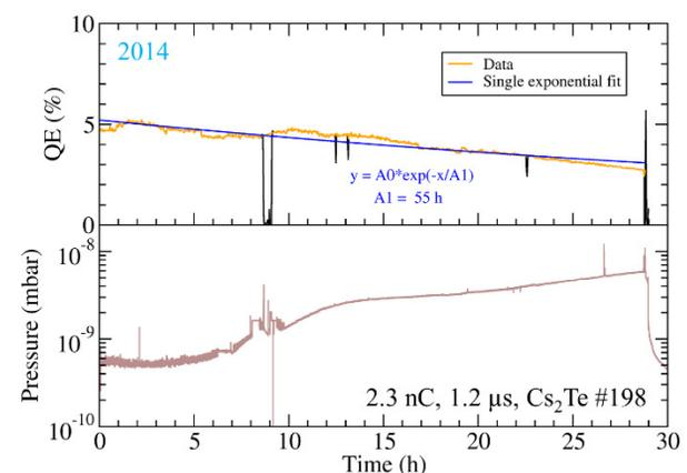
Figure 1: Pressure increase and short cathode lifetime measured in 2014.
