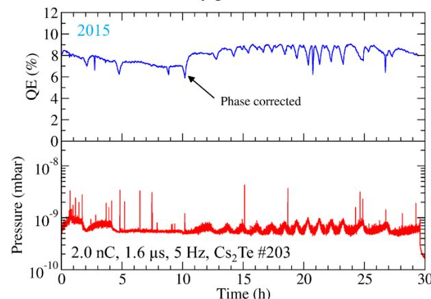
Figure 4: Lifetime measurement of Cs<sub>2</sub>Te cathode #203 with 2.0 nC/bunch, 1.6 μs train length and 5 Hz macro-pulse repetition rate.
