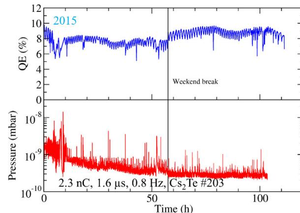
Figure 3: Lifetime measurement of Cs<sub>2</sub>Te cathode #203 with 2.3 nC/bunch, 1.6 μs train length and 0.8 Hz macro-pulse repetition rate.
