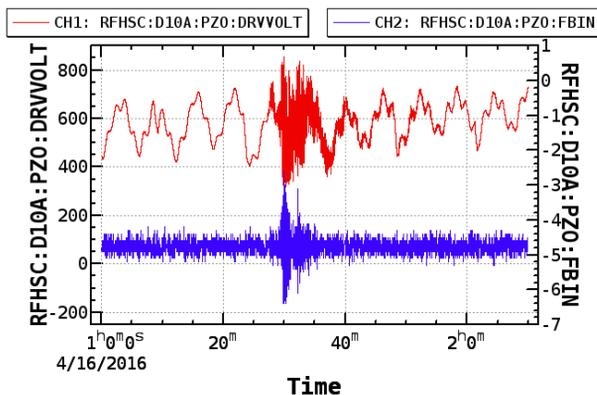
Figure 9: Variation of the tuner voltage (red) position (blue).
