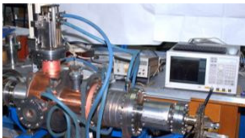
Figure 2: Photo of the harmonic cavity on bench.
