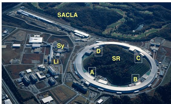
Figure 1: SPring-8 Accelerator complex. SR: Storage ring, Sy: 8 GeV Booster synchrotron, Li: 1 GeV Injector linac, A-D: RF stations, and SACLA: 8 GeV XFEL.
