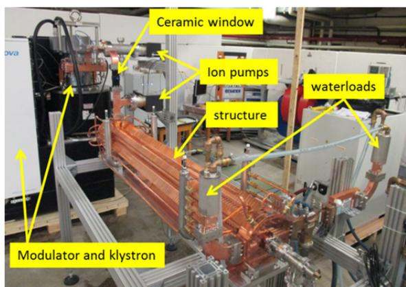
Figure 9: C-band structure under high power test.
