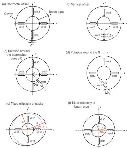
Figure 2: Simulated misalignments: (a) Slot1 offset in  $x$  by  $\Delta x$ . (b) Slot1 offset in  $y$  by  $\Delta y$ . (c) Slot1 rotated around the cavity axis by  $\Delta\Theta_c$ . (d) Slot1 rotated around its axis by  $\Delta\Theta_g$ . (e) Elliptical cavity rotated by  $\Delta\Theta_c$ . (f) Elliptical beam pipe rotated by  $\Delta\Theta_b$ .
