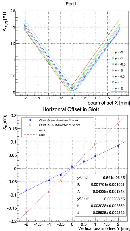
Figure 7: Top: horizontal beam position sensitivities with fixed vertical beam offsets in the Port1. A fitting function  $a|x - b| + c$  is applied. Bottom: Cross-couplings in horizontal misalignment in Slot 1. Horizontal offsets in Slot1 are chosen by -8 % and -16 % of dimension of the slot.
