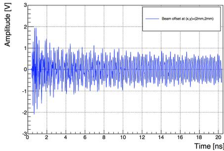
Figure 3: The port signal simulated by GdfidL for the original geometry.
