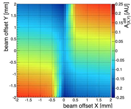
Figure 6: Normalised difference amplitude in case of the horizontal offset of the slot.
