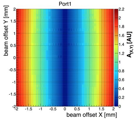
Figure 5: Normalised amplitude in the original geometry.
