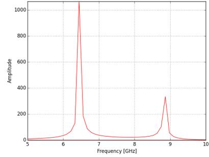
Figure 4: FFT of the port signal. The second peak corresponds to a quadrupole mode.
