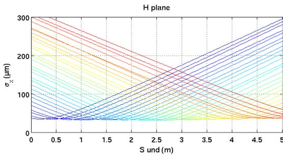
Figure 2: Horizontal slice beam envelopes along 5 m of undulator. Colours according to the energy deviation as figure 1.
