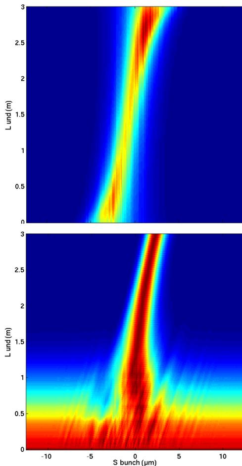
Figure 5: Example of transverse electron density (up) and according FEL peak power (down) along the 3 m undulator with the chromatic matching.
