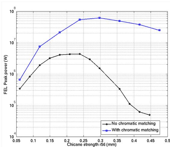
Figure 4: Output FEL peak power comparison versus chicane strength.
