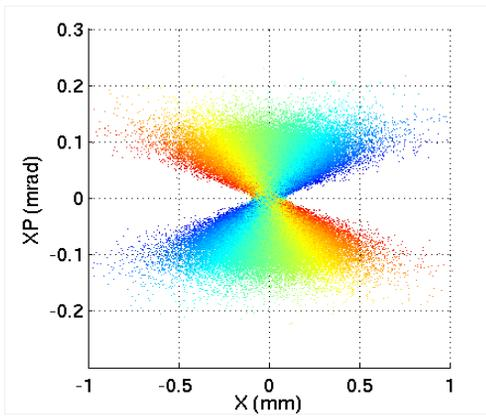
Figure 1: Horizontal phase space at undulator centre. Colours according to the energy deviation.
