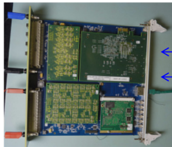
Correcor Power Supply Controller (EPICS IOC with Fast Setting FPGA Design)
