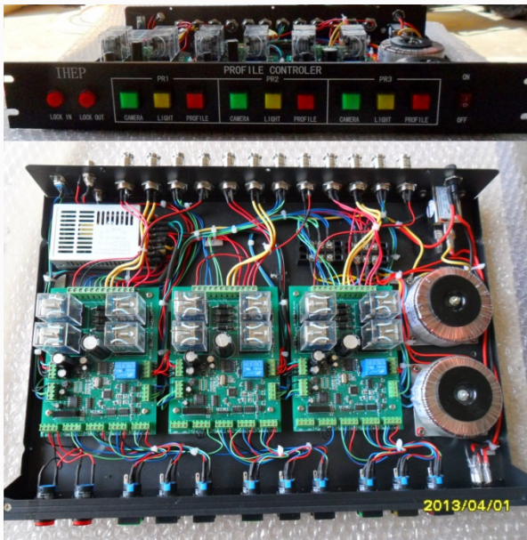
PR electronics and control unit
