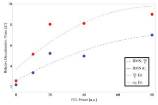
Figure 4: Variation in optimal return linac relative phase vs. increasing FEL induced energy spread.
