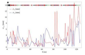
Figure 7: Transverse beam properties for the 2-loop ALICE ERL at 60 pC.
