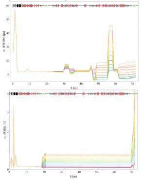
Figure 2: Longitudinal properties of the ALICE machine for various linac off-crest phases from  $0^{\circ}$  (Red) through  $8^{\circ}$  (green) to +16° (Orange), and at a 60 pC bunch charge.
