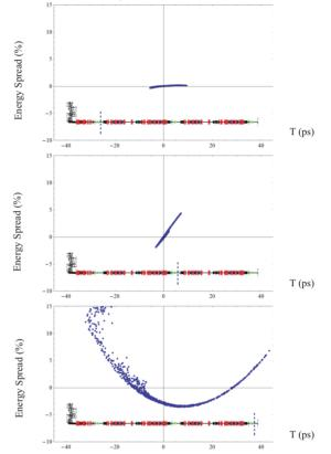
Figure 8: Longitudinal phase space at the exit of the  $2^{nd}$  linac cavity for each of the 3-passes at 60 pC.
