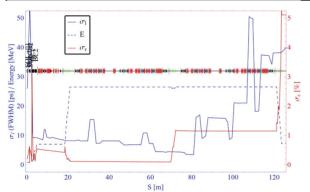
Figure 6: Longitudinal beam properties for 2-loop ALICE ERL at 60 pC.
