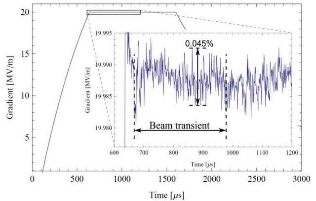
Figure 5: Vector sum gradient [MV/m] versus time [μs] after automated generation of beam FF table.
