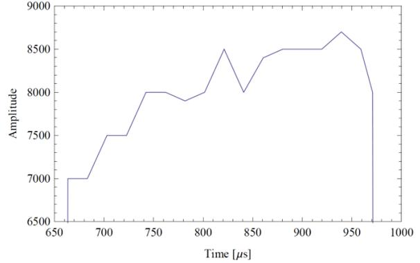
Figure 4: Amplitude versus time [μs] of automatically generated beam FF table.
