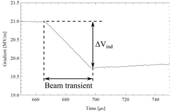
Figure 2: Cavity 1 gradient [MV/m] versus time [μs] during the flattop covering the beam transient, during which beam loading induces the gradient drop  $\Delta V_{ind}$ .
