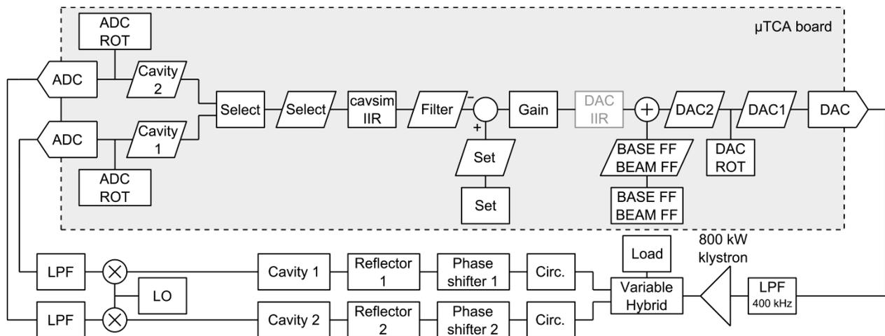
Figure 1: Schematic of the digital LLRF feedback loop controlling two superconducting cavities at STF. Hardware and software components are represented by squares, data channels accessible on the  $\mu$ TCA board via EPICS by rhombi.
