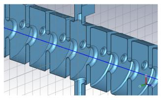
Figure 6: Cut-plane view of the cell-shapes and coupler design.
