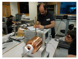
Figure 3: Prototype cavity tuning range evaluation.
