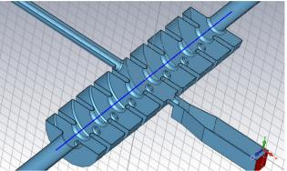
Figure 1: View of the final cavity design, showing the input coupler and dummy waveguide.
