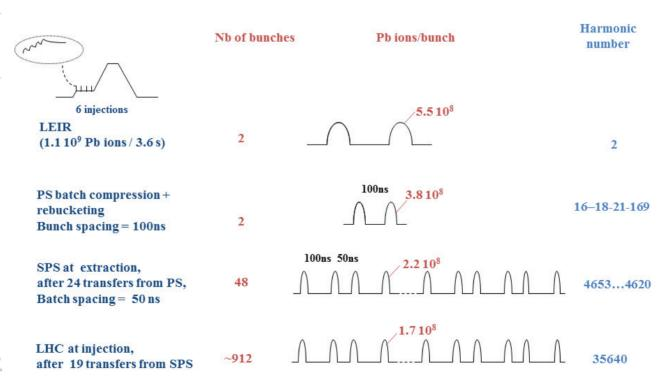
Figure 2: Alternating 100/50 ns spacing scheme, with 24 PS injections into the SPS. The beam intensities correspond to the ones achieved for the p-Pb run in 2013.
