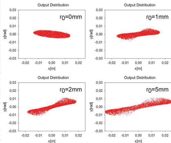
Figure 4: Output phase space distributions of the  $\text{He}^{1+}$  at 14keV. The electron free zone is limited by the variable radius  $r_0$ .
