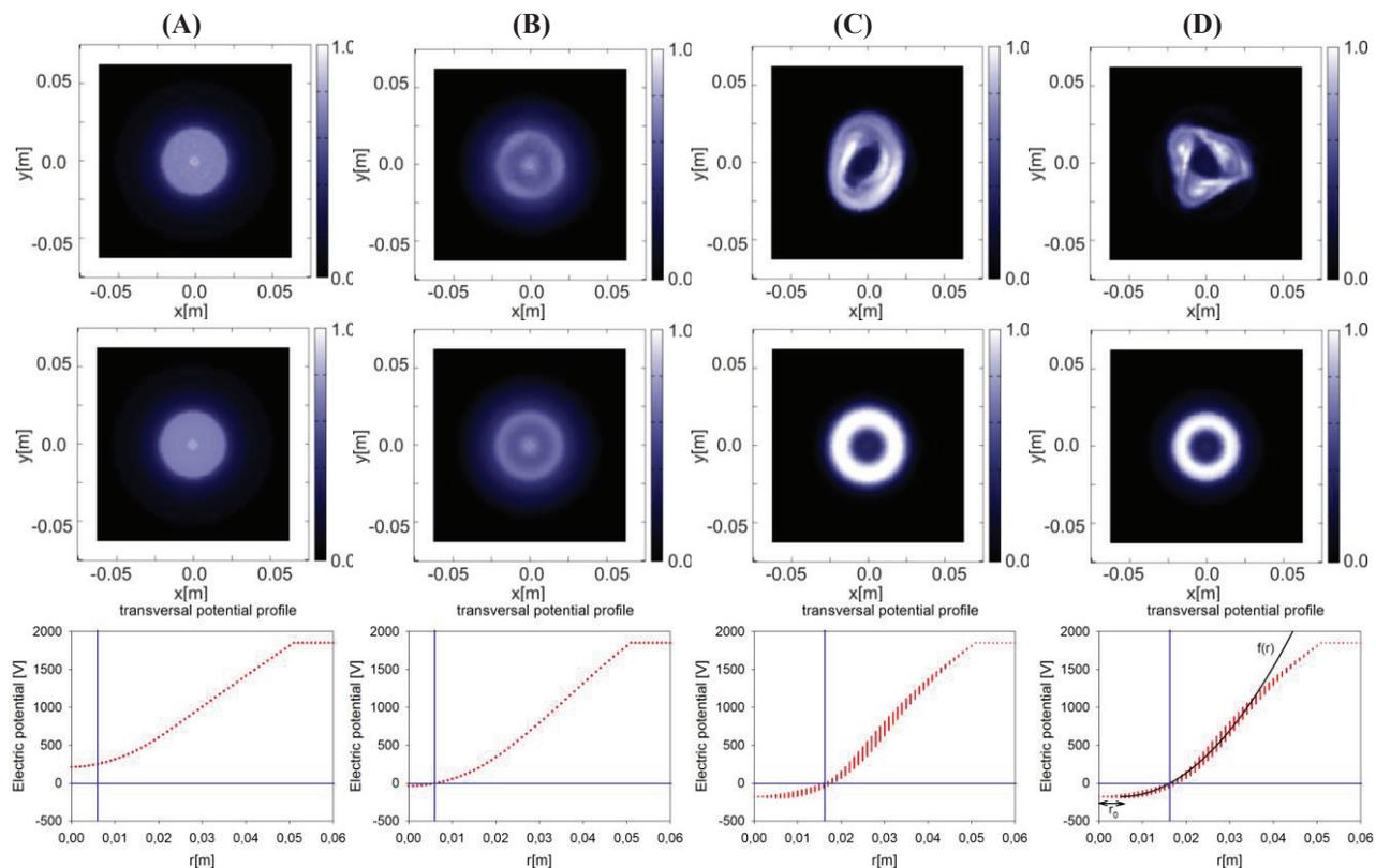
Figure 3: Example of simulated four different (A, B, C, D) non-neutral plasma states within the Gabor lens. In the first row, the  $z$ -integrated electron density is depicted, at  $t=1\mu\text{s}$ . In the second row the effective density averaged over 1 ms is shown. In a third row the according transverse potential profile in the centre plane of the Gabor lens at  $t=1\mu\text{s}$  is displayed.
