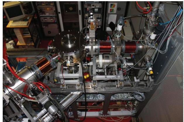
Figure 2: LEBT test setup consisting of a volume type ion source, an array of three Gabor lenses and a 45° electrostatic deflector.
