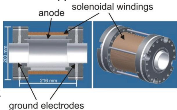
Figure 1: Layout of the Gabor lens designed and used at IAP Frankfurt.
