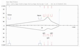
Figure 3: Transverse envelops of the beam along one beam line (horizontal plane on top, vertical plane on bottom).
