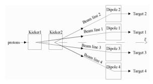
Figure 2: Beam switchyard principle.
