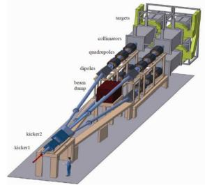
Figure 4: Beam switchyard layout.
