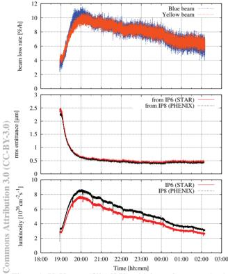
Figure 1: U–U store (fill 16858) with beam loss rates (top), rms emittances (middle), and luminosities (bottom). The reduction in the emittances and the corresponding increase in the luminosity is due to stochastic cooling.
