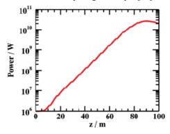
Figure 4: Power growth in XFELO seeded high-gain FEL.
