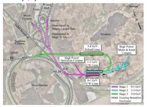
Figure 1: Layout of Project-X configuration.
