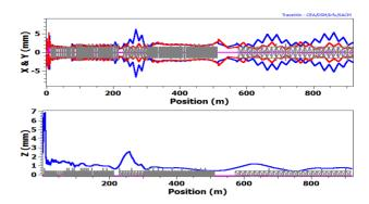
Figure 3:  $1 \times \sigma_{rms}$  beam envelopes. Top: transverse (*x*-blue, *y*-red). Bottom: longitudinal.
