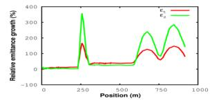
Figure 4: Relative emittance growth along the linac in longitudinal (green) and transverse (red) plane.
