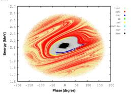
Figure 5: Longitudinal acceptance of baseline design at different locations along the CW linac.
