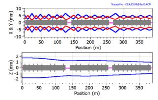
Figure 7:  $3\sigma_{rms}$  beam envelopes. Top: transverse (*x*-blue, *y*-red). Bottom: longitudinal.
