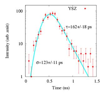
Figure 2: Measured positron lifetime spectrum of yttriastabilized zirconia (YSZ). Solid curves are least squares fitting curves of data points derived from Eq. (4). Positron lifetime for YSZ is evaluated as  $162\pm18$  ps.
