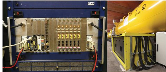
Figure 1: MTCA.4 crate with radiation shielding at DESY’s free electron laser facility FLASH.
