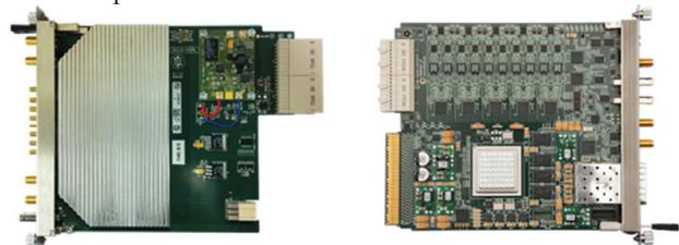
Figure 2: Pair of MTCA.4 boards (RTM left, AMC right)
