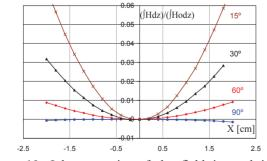
Figure 10: Inhomogeneity of the field integral in the bump magnet normalized on field integral in the centre for various phases of a current pulse.
