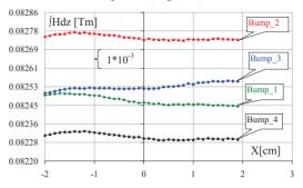
Figure 11: Integrated field value of the bump  $1 \div$  bump 4 with the vacuum chamber.
