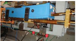
Figure 1: Top view of the injection septum magnet.
