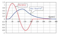
Figure 6: The magnetic field in injection magnet and stray a field in the vacuum chamber vs time.
