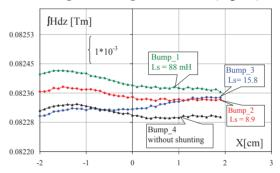
Figure 12: Integrated field value of bump  $1 \div$  bump 4 with the vacuum chamber and with shunting inductance.
