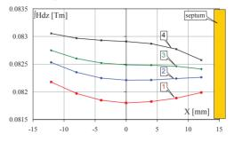
Figure 5: Inhomogeneity of the field integral in the magnet during various moments of time.
