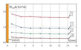
Figure 7: Distribution of the stray field in the booster vacuum chamber at the various moments of time. 1 – Extraction septum t=75  $\mu$ s (Hin = 0.8 T),
