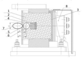
Figure 2: Cross-section view of the injection septum magnet.
