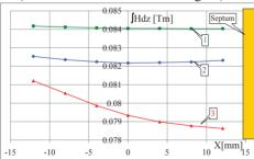
Figure 4: Distribution of the field integral in the aperture of the injection septum.
