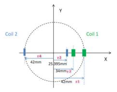
Figure 1: Measurement coil schematic diagram.
