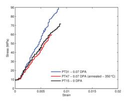
Figure 5: Annealing effect on tensile properties of POCO.
