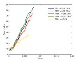
Figure 4: Stress strain curves for irradiated IG-430 at varying DPA levels.
