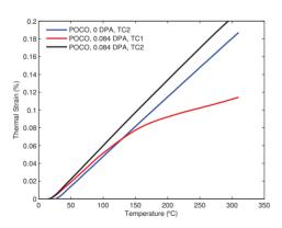
Figure 2: Dimensional changes in un-irradiated and irradiated POCO graphite over two thermal cycles.
