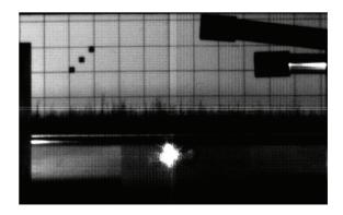
Figure 5: Powder erruption at 37 ms after beam impact: the powder has reached its peak position about 6 mm above the initial maximum position.
