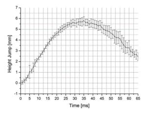
Figure 6: The disruption height as a function of time after beam impact of  $2 ext{ } 10^{11}$  protons/pulse.
