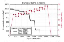
Figure 6: Beam scraping within one SPS cycle in steps of 200 ms separated by 200 ms.
