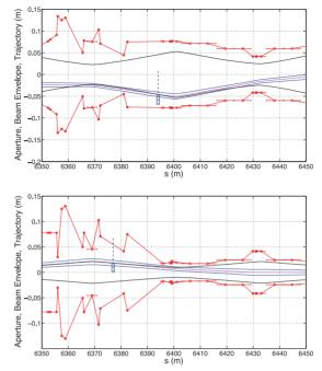
Figure 2: Horizontal (top) and vertical (bottom) machine apertures, beam envelopes and orbits vs. longitudinal position along the SPS.
