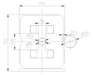
Figure 3: Preliminary mechanical design for the new vertical bumpers.
