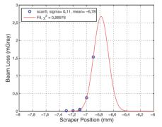
Figure 5: Beam profile acquired by the operational scraper scan after the beam cleaning onto the TPSG; an orbit amplitude of 36 mm and 1.11 mrad was used.
