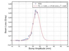
Figure 4: Beam profile measured using the TPSG mask.
