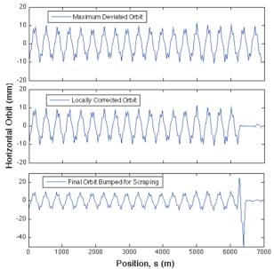
Figure 1: Variation of the horizontal orbit as a function of the position along the SPS.
