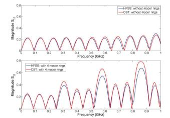
Figure 2: Magnitude of  $S_{11}$  predicted by HFSS and CST MS, for striplines without (top) and with (bottom) Macor rings.
