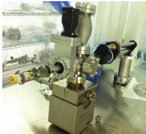
Figure 4: Photograph of the load-lock chamber with the magazine in the foreground. Two sets of pucks are mounted on the magazine.
