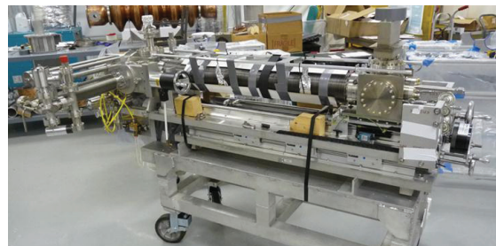
Figure 9: Photograph of the transport cart, baked and ready to be attached to the gun.
