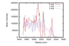
Figure 7: The beam intensity along radius of the last few turns for 0, 1 and 5 mA beam current.
