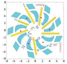
Figure 1: The updated layout sketch of the 800 MeV cyclotron solution, including injection and extraction elements (MCA: main cavity, FCA: flat-top cavity, FDM: focusing doublet, BM: bending magnet, MIC: magnetic injection channel, EIC: electric injection channel, FM: focusing magnet, EEC: electric extraction channel).
