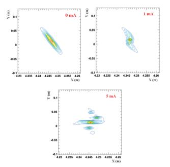
Figure 8: Top view of the bunch distribution at 0° azimuth of turn 50 in global coordinates for 0, 1 and 5 mA beam current scenarios.
