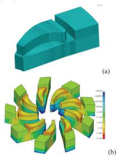
Figure 2: (a) The 1/8 model of the main magnet; (b) the magnetic flux intensity distribution on the main magnet.
