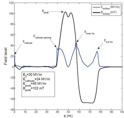
Figure 4: Surface electric and magnetic field of the gun cavity including cathode stock and choke cell normalized to maximum on-axis field  $E_0$  of 30 MV/m versus surface path length  $s$  starting from the cathode, through the Petrov/choke filter part and finally the cell surfaces.
