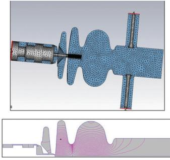
Figure 2: Setup of the cavity geometry for RF simulation with CST MWS and Superfish including the Choke cell and Petrov filter for studies of cathode retraction.
