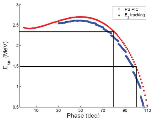
Figure 5: Comparison of kinetic energy versus emission phase at  $E_0=30$  MV/m for several bunches (blue) using a simple tracking program compared to CST's PIC Solver. The black lines denote a possible phase and resulting energy range of field emitted dark current near the cathode.
