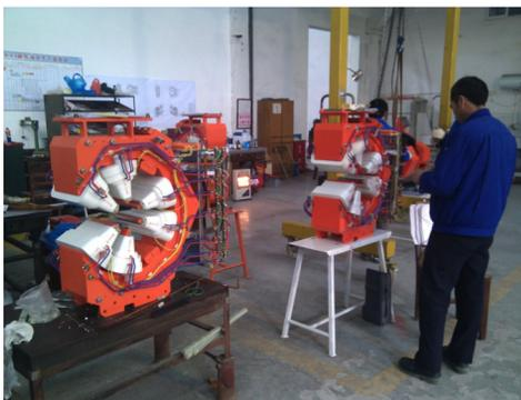
Figure 3: Assembly of magnets at SINAP.
